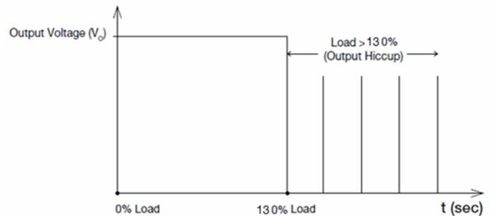
Additionally, if the  $I_o$  is  $< 135\%$  but  $> 110\%$  for a prolonged period of time (depending on the load), the Over Temperature Protection (OTP) will be activated due to high temperature on critical components. The power supply will then go into hiccup mode until the fault is removed; and, the input voltage is removed, then reapplied.
